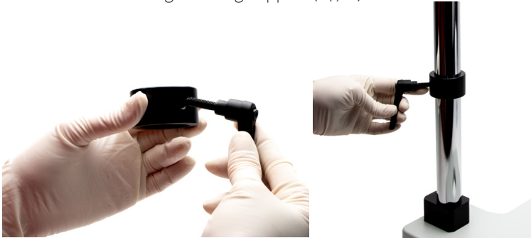
Fig. 6—(Left) Screw the clutch handle into the threaded hole in the side of the guard ring. Fig. 7—(Right) Slide the guard ring over the top of the vertical post.
